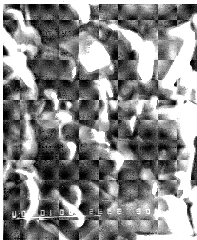
Fig. 4. Microstructure of piperazine malonate synthesized by OSHS
